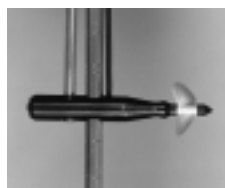
2100-TSR Adapter for using optical sensor on a USGS style wading rod
